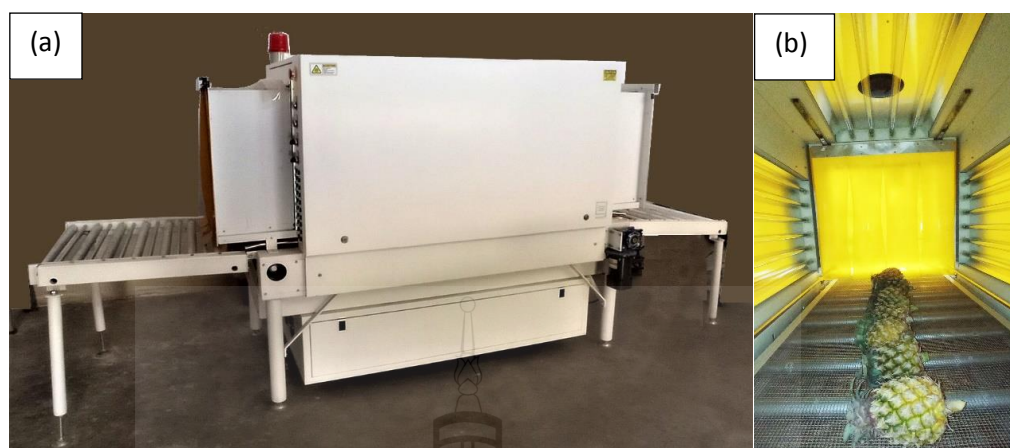
Figure 3.2 UV-C chamber (a) External design and (b) Internal design
