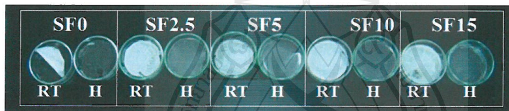
Fig.4.4 The SF/CAB blend films containing 0% (SF0), 2.5% (SF2.5), 5% (SF5), 10% (SF10) and 15% (SF15) (w/w) SF contents. All films (10% total mass content) were casted in a 15:85 (formic acid/acetone) mixture solvent. The drying conditions used were at room temperature (RT) and at elevated temperature (50°C) in the oven (H).
