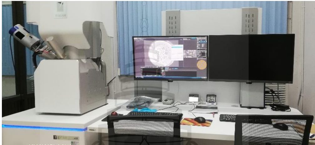
Figure 3.11 Scanning electronic microscope, model MIRA of TESCAN company, Czech Republic
