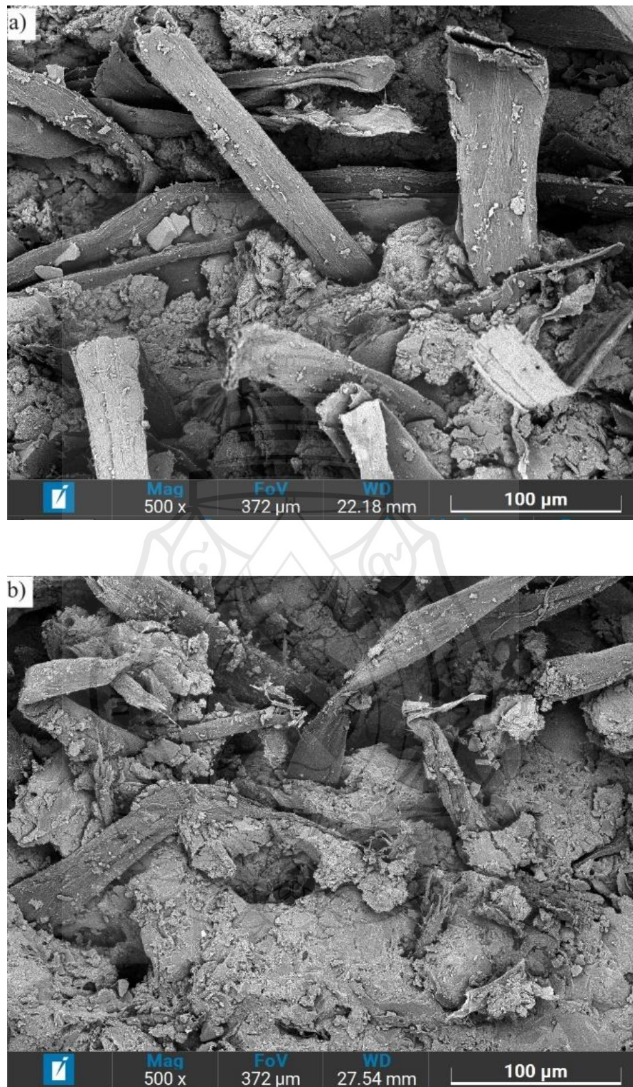
Figure 7.6 Micrographs of fracture surfaces of EFC: a) fiber pull out mode and b) fiber failure mode
