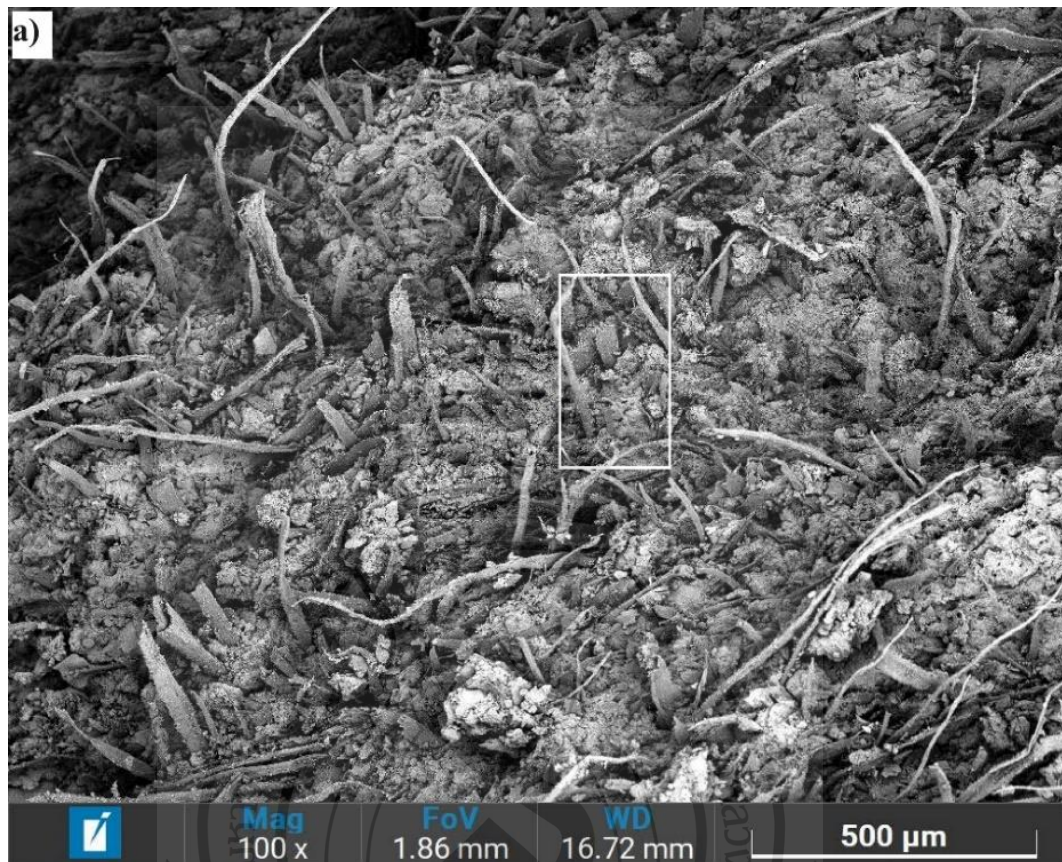
Figure 5.5 SEM photographs of surface fractures of 550 mL CSF RPBCC: a) 100x and b) 500x magnitude
