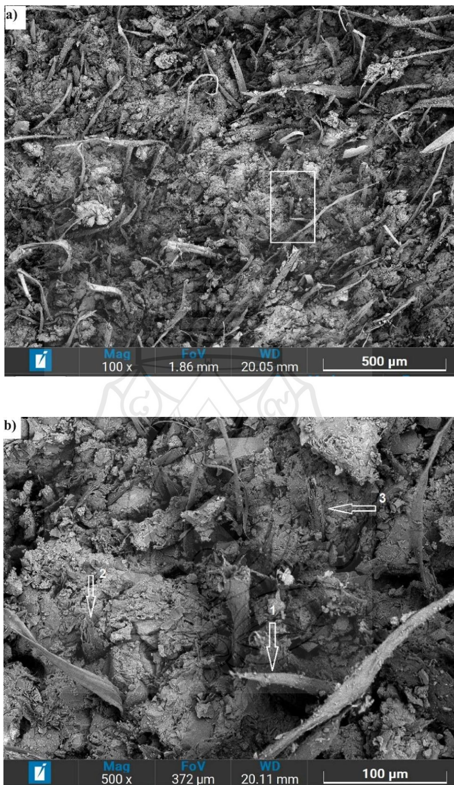
Figure 5.6 SEM photographs of surface fractures of 400 mL CSF RPBCC: a) 100x and b) 500x magnitude
