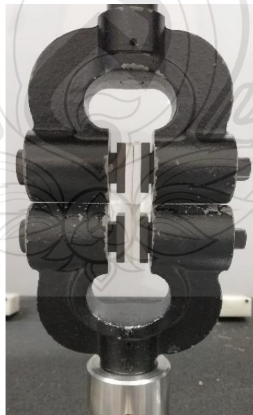
Figure 3.15 Cramping jaw for the zero-span test of handsheet paper
