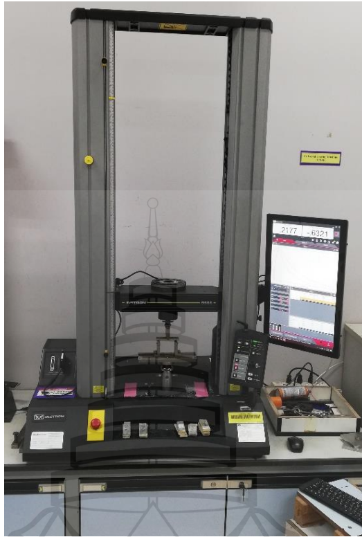
Figure 3.14 Universal testing machine (Instron type 5632)
