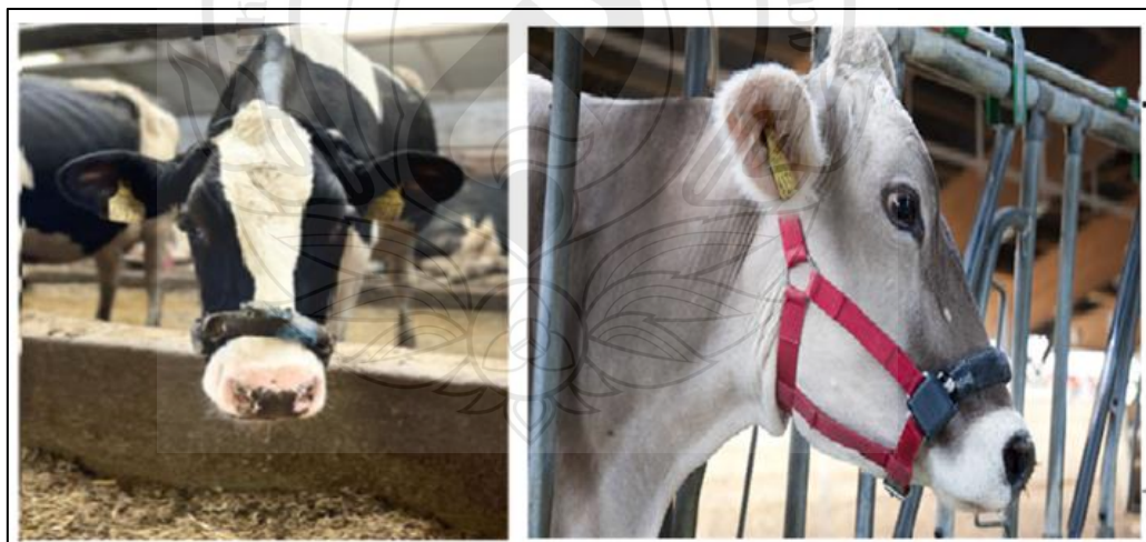
Figure 2.10 Cow with RumiWatch Noseband Sensor (front and side view) (RWS; ITIN + HOCH GmbH, Feeding Technology, Liestal, Switzerland)
