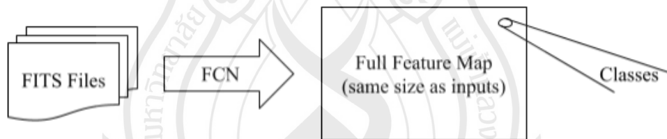
Figure 2.4 Fully convolutional network procedures
