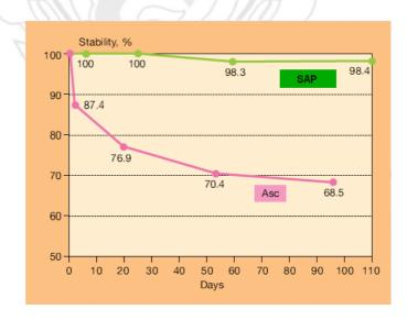
Figure 2.11 Stability of SAP and ascorbic acid (Asc)  $\,$  2% in water,  $\,$  20°C, pH  $\,$ 7  $^{13}$
