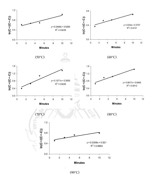
Figure C.9 First order plot for GC extraction from green tea at various time and temperatures
