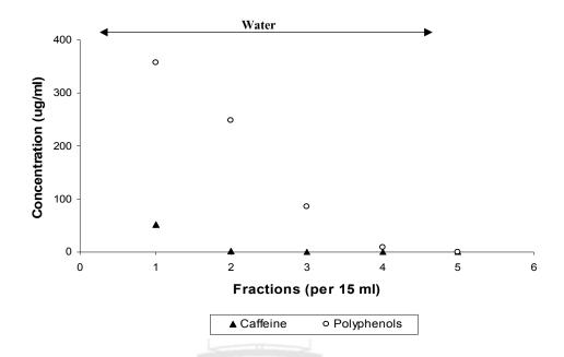
**Figure 4.22** Peak profile of total polyphenols and caffeine contents from nylon 6 with medium sized column
