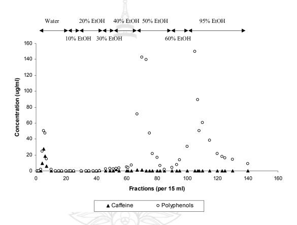
**Figure 4.24** Peak profile of total polyphenols and caffeine contents from polyamide 6 with medium sized column and gradient elution
