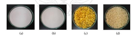
**Figure. 4.14** Physical appearance of polyamide 6 (a), amberlite XAD7HP (b), poly (dimmer acid-co-alkyl polyamine) (c), and nylon 6 (d)
