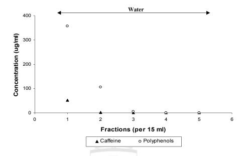
Figure 4.20 Peak profile of total polyphenols and caffeine contents from poly (dimmer acid-co-alkyl polyamine) with medium sized column
