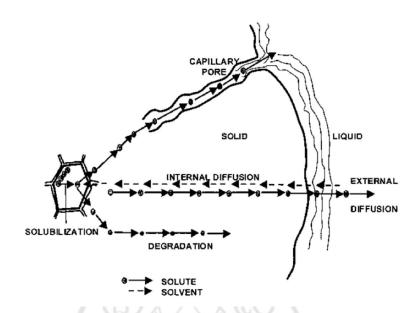
**Figure 2.12** Schemes of the main steps in solvent extraction of solid particle Source: Aguilera (2003)
