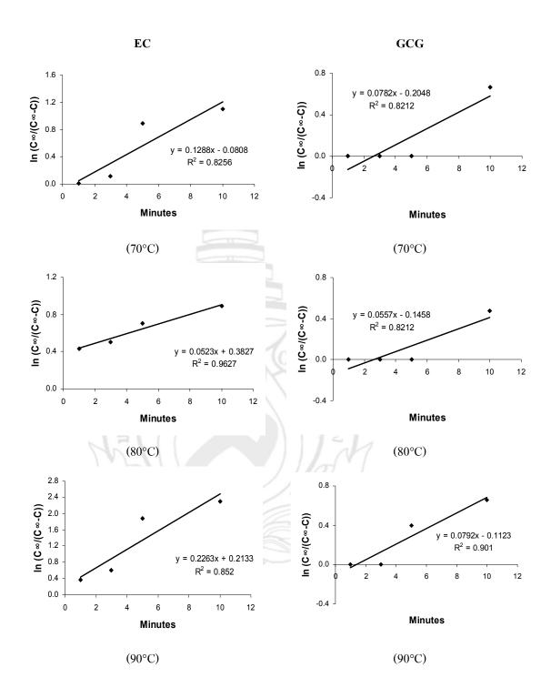
**Figure D.5** First order plot for EC and GCG extraction from green tea at various time and temperatures
