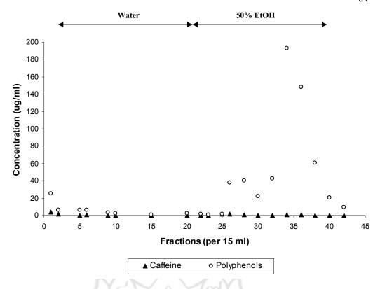
**Figure 4.15** Peak profile of total polyphenols and caffeine contents from polyamide 6 with medium sized column
