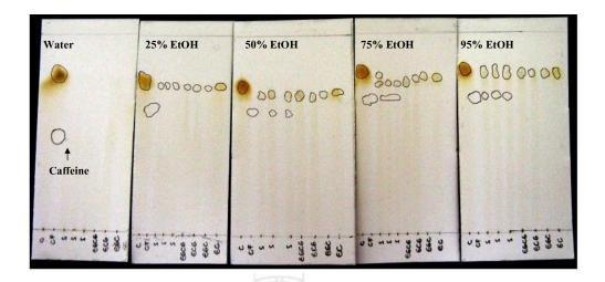
**Figure. 4.13** Thin layer chromatography of green tea extract, caffeine and catechins compounds (from left to right: C, caffeine, sample, sample, EGCG, ECG, EGC and EC)
