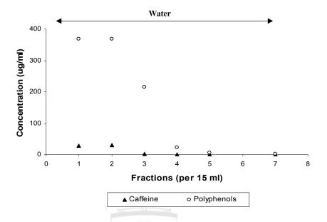
**Figure 4.21** Peak profile of total polyphenols and caffeine contents from poly (dimmer acid-co-alkyl polyamine) with small sized column
