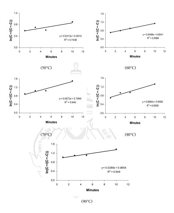
Figure C.10 First order plot for C extraction from green tea at various time and temperatures
