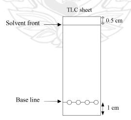
Figure 3.2 TLC Aluminium Sheet
