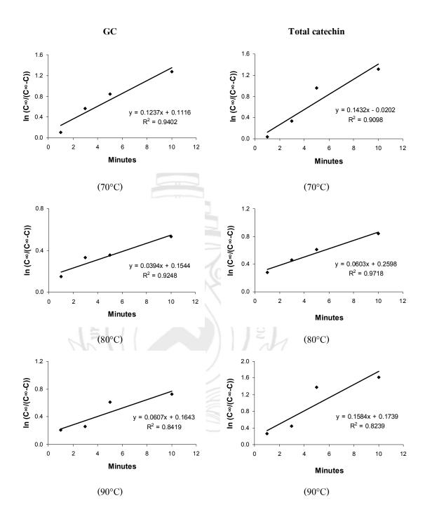
**Figure D.6** First order plot for GC and total catechins extraction from green tea at various time and temperatures
