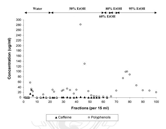
**Figure 4.16** Peak profile of total polyphenols and caffeine contents from polyamide 6 with small sized column
