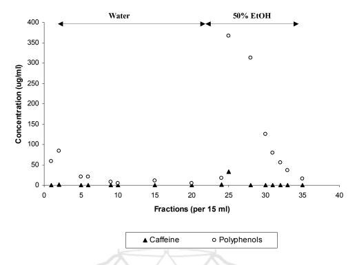
**Figure 4.18** Peak profile of total polyphenols and caffeine contents from amberlite XAD7HP with medium sized column
