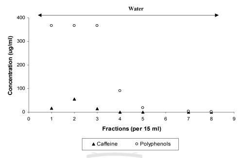
**Figure 4.23** Peak profile of total polyphenols and caffeine contents from nylon 6 with small sized column
