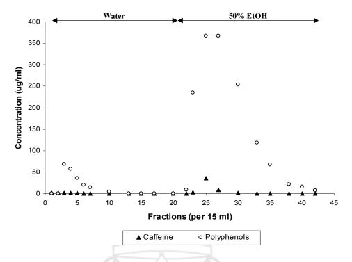
**Figure 4.19** Peak profile of total polyphenols and caffeine contents from amberlite XAD7HP with small sized column
