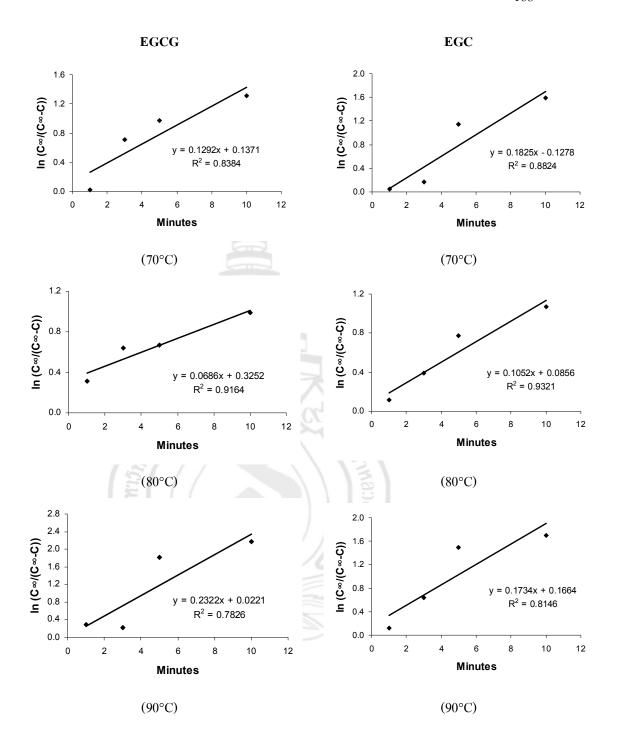
**Figure D.4** First order plot for EGCG and EGC extraction from green tea at various time and temperatures
