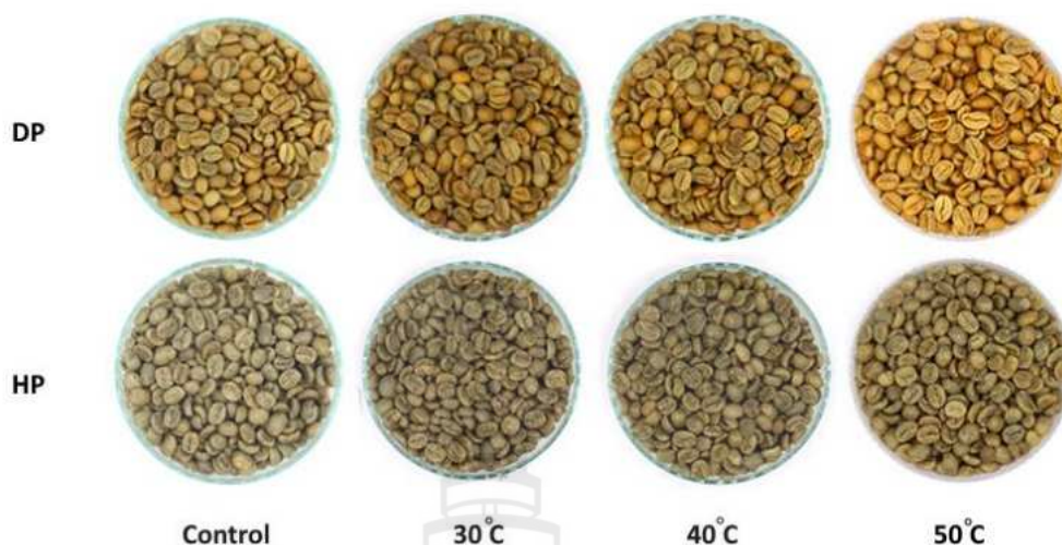
Figure 6.2 Green Coffee Bean Storage in GrainPro® Bags after 20 Days under Accelerated Storage Condition
