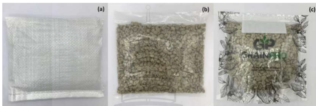
Figure 5.1 Packaging for GCB Storage (a) Plastic Woven Bag (PW), (b) Low-Density Polyethylene Bag (LDPE) and (c) GrainPro® (GP)
