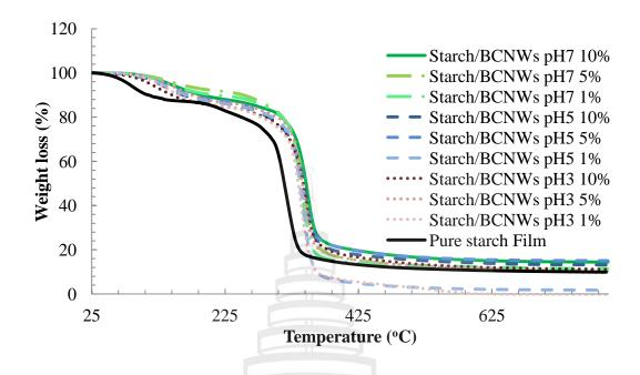
**Figure 4.13** TGA Curves of the Pure Starch Film and Bionanocomposite Films Reinforced with BCNWs of pH 3, 5 and 7 (with Varied Contents of 1, 5 and 10 wt%)
