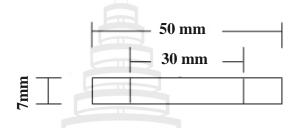
Figure 3.4 Illustration of Tensile Specimens
