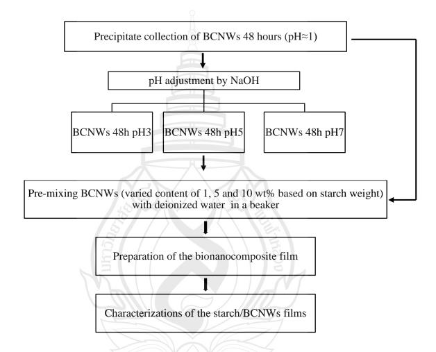
Figure 3.3 Flow Chart of Preparation of the Bionanocomposite Films
