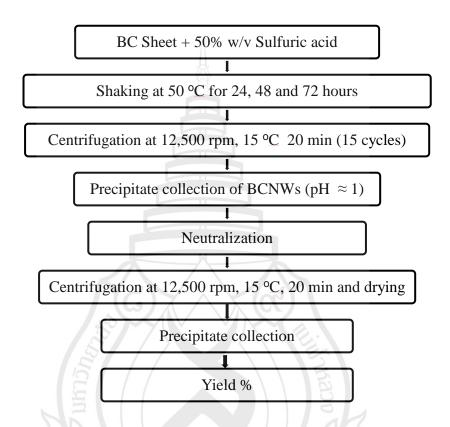
Figure 3.1 Flow Chart of Bacterial Cellulose Nanowhiskers (BCNWs) Preparation
