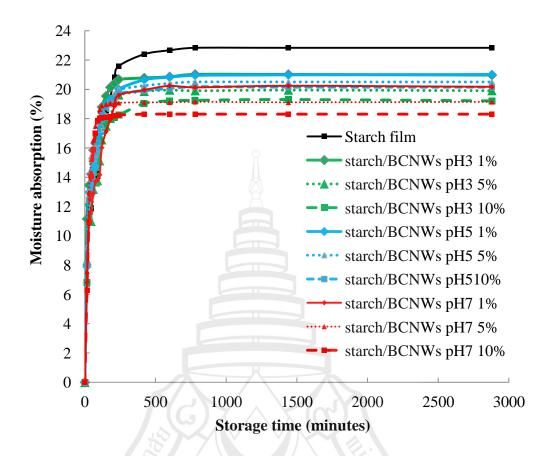
**Figure 4.12** Moisture Absorption (at 75% RH) as a Function of Storage Time of the Pure Starch Film, and Bionanocomposite Films Reinforced with BCNWs of pH 3, 5 and 7 (with Varied Contents of 1, 5 and 10 wt%)
