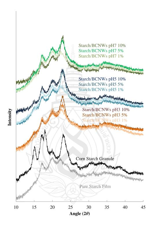
**Figure 4.6** X-ray Diffraction Patterns of the Corn Starch Granule, Pure Starch Film and Bionanocomposite Films Reinforced with BCNWs of pH 3, 5 and 7 (with Varied Contents of 1, 5 and 10 wt%)
