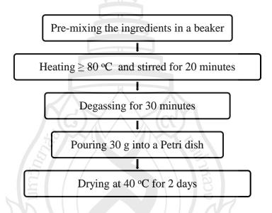
Figure 3.2 Flow Chart of Preparation of Standard Films
