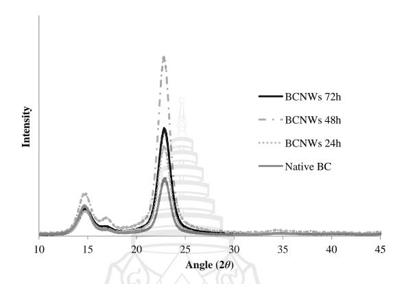
**Figure 4.2** X-ray Diffraction Patterns of the Native Bacterial Cellulose (BC) and the Obtained Nanowhiskers (BCNWs) after Acid Hydrolysis Time of 24, 48 and 72 Hours (BCNWs 24h, BCNWs 48h and BCNWs 72h, respectively)
