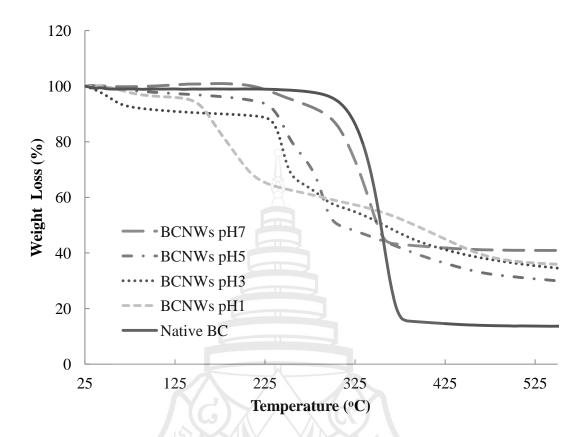
**Figure 4.4** TGA Curves of the Native BC, BCNWs after Acid Hydrolysis Time of 48 Hours (BCNWs pH 1) and BCNWs 48 Hours with pH Adjusted to 3, 5 and 7 (BCNWs pH 3, BCNWs pH 5 and BCNWs pH 7, respectively)
