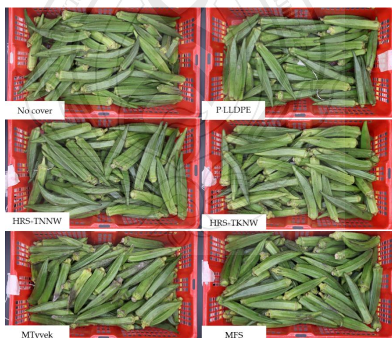
Figure 4.13 Okra from Six Treatments after Simulated Storage at 18 °C for 48 h and Simulated Transportation at 30 °C for 15 h
