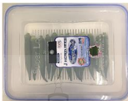
Figure 2. Okra pods packed in a plastic food container for respiration rate measurement by a closed system.
