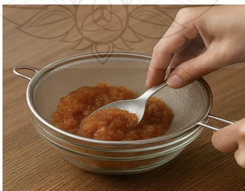
Figure 3.3 Peach gum matrix after boiling, drained with a standard strainer and homogenized before analysis
